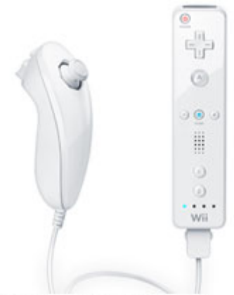
Wii's controller uses MEMS sensors and wireless technology to detect the motion and tilt of a player's hand in all three dimensions and convert it into game action.
