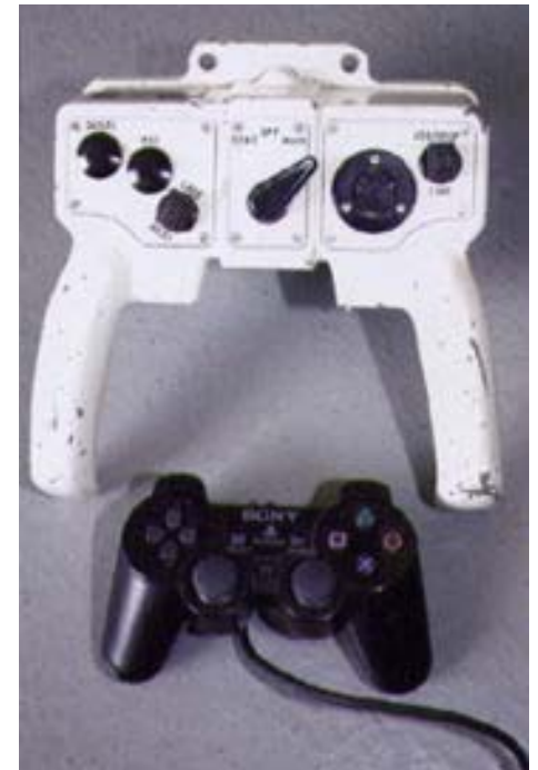
☞ Dualshock controller compared to gun controller of the British Challenger 2 main battle tank
